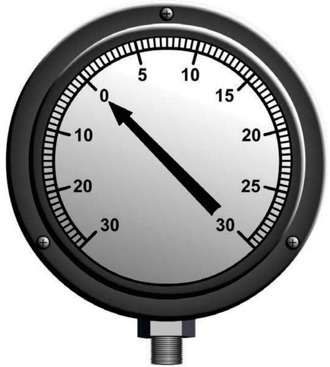
Figure 11-5 — Compound Bourdon-tube gauge.
