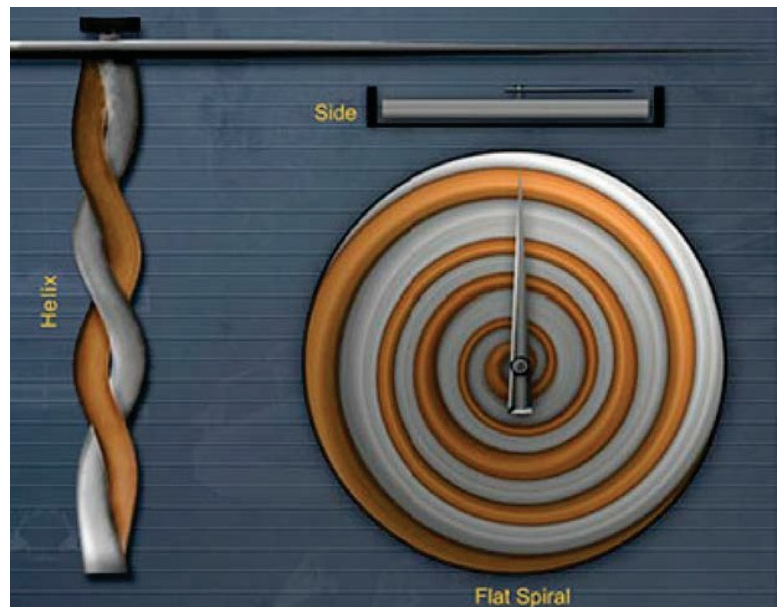
Figure 11-12 — Bimetallic thermometer (flat, spiral strip).
