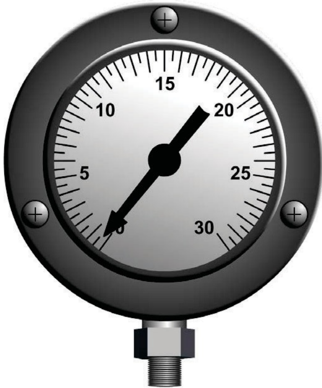
Figure 11-4 — Bourdon-tube vacuum gauge.
